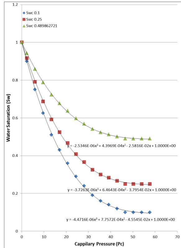
Figure 9. Cross Plot of Water saturation vs Capillary Pressure
