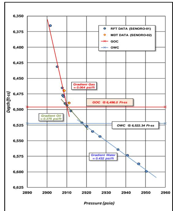
Figure 7. Fluid Contact Determination
