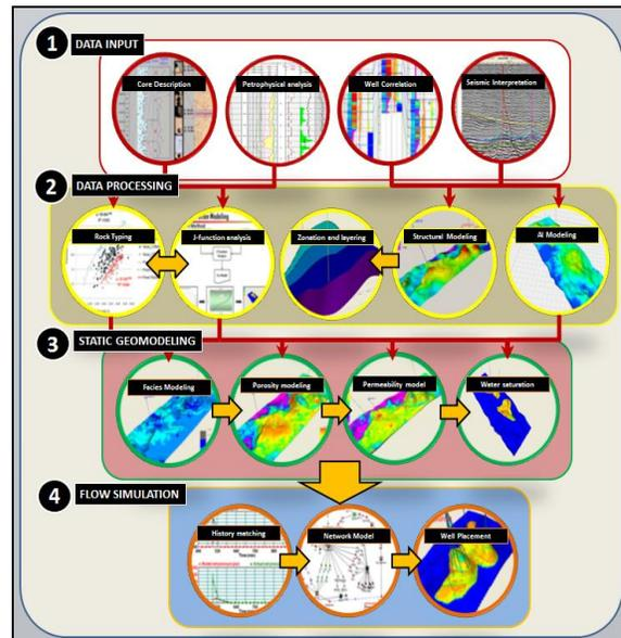
**Figure 5. General workflow of Senoro static geologic modeling**
